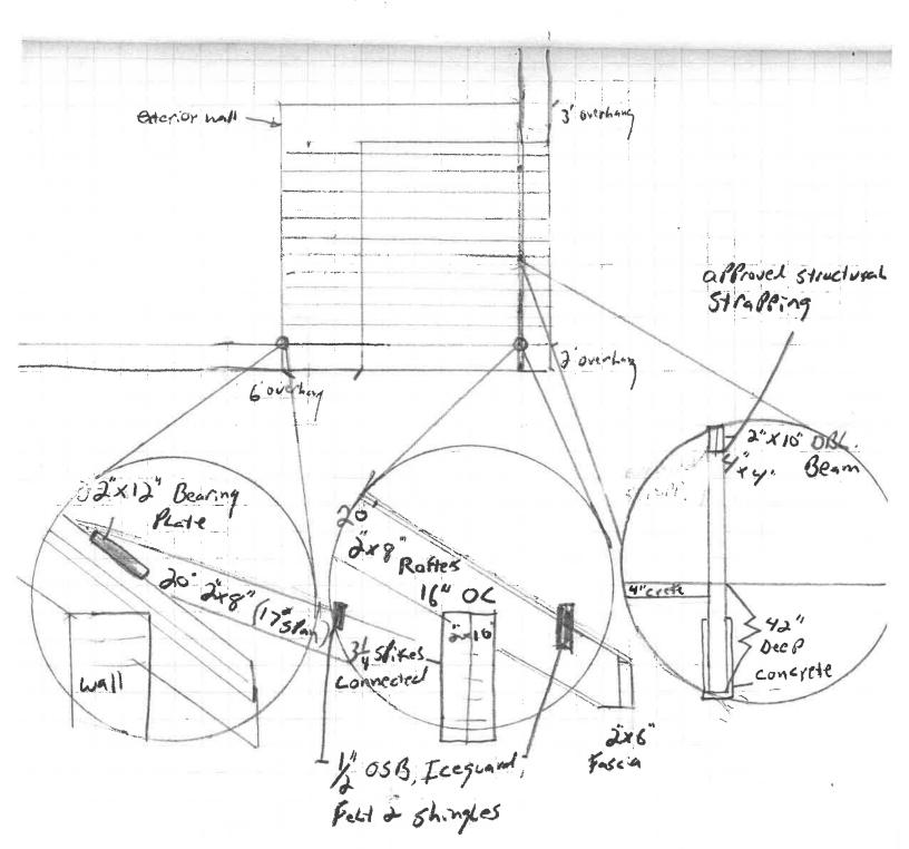
17' - 2'x8' Maker Stans 16"06. Bearing on a"x12" Place over subbutting his of & 2"x10" LBL Beam (\$ 6" Between Pusts).
